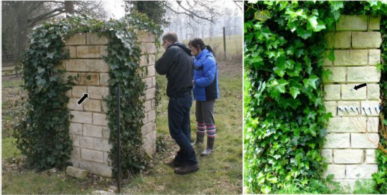
Figure 5. Test walls constructed of Elm Park Limestone and lime mortar, Wytham Woods, Oxfordshire. The structure had four faces (north, east, south and west facing) 1.2 m wide and 2 m high. Ivy was allowed to establish on one half of each face, allowing controlled comparisons between exposed and ivy covered stone. Arrows indicate the position of temperature loggers.
